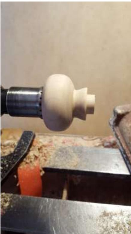
It was tiring to make one knob at a time so I made several and dyed the white maple different colors. I also used natural woods for the knobs in the picture below.
