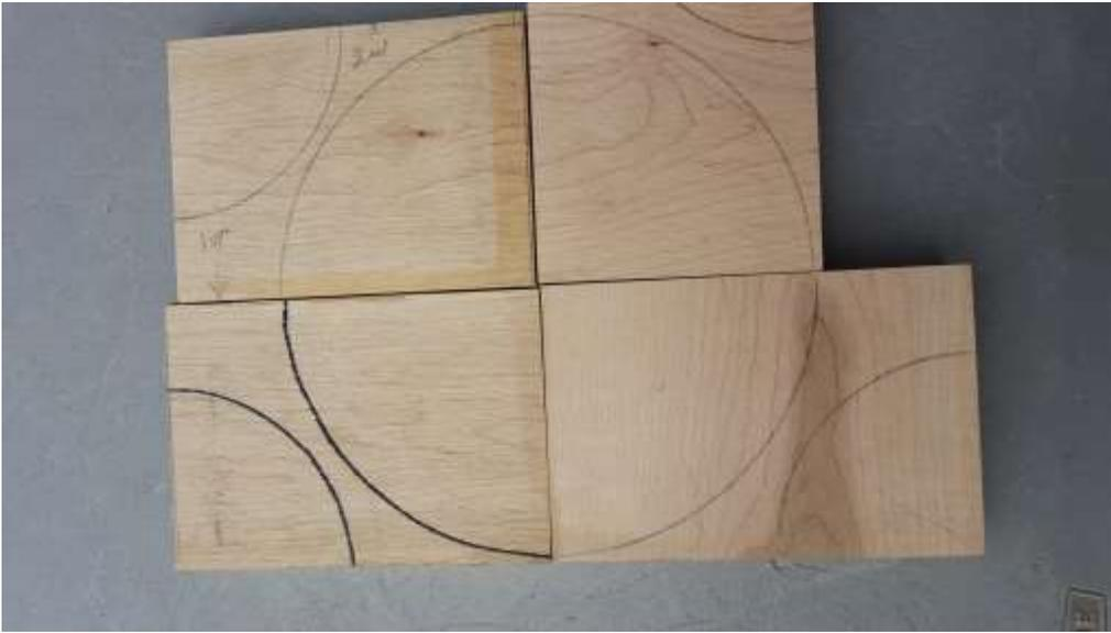
Cut the large and smaller quarter's out using the band saw. The picture below shows what the large and smaller quarter would look like.
