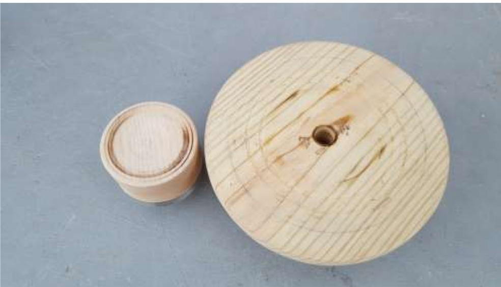
Place the wood that has been cut round on a bandsaw between the wooden disk and tailstock. I use the Hunter tools to true it up and also true the face towards the tailstock live center. You of course can use any tool of your choosing.
