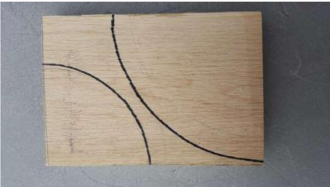
Use a compass and mark quarter circles, one for the Stronghold chuck 4¼ inches and the smaller quarter for the talon chuck at 3 inches as marked above. Do this on all four pieces of Maple stock.
