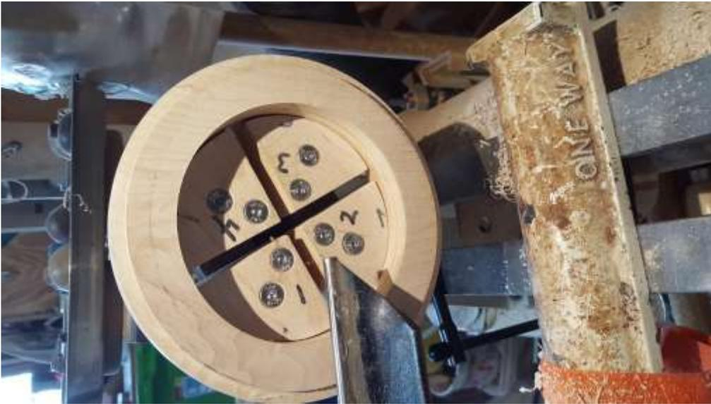
Clean up the inside and sand this area. Shape the outer area for the top of the box.
