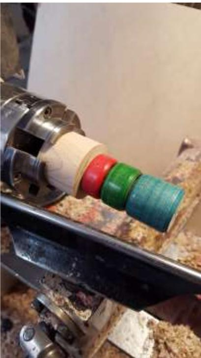
The picture below shows a cut bead in the wood which will be the top of the finished knob.
