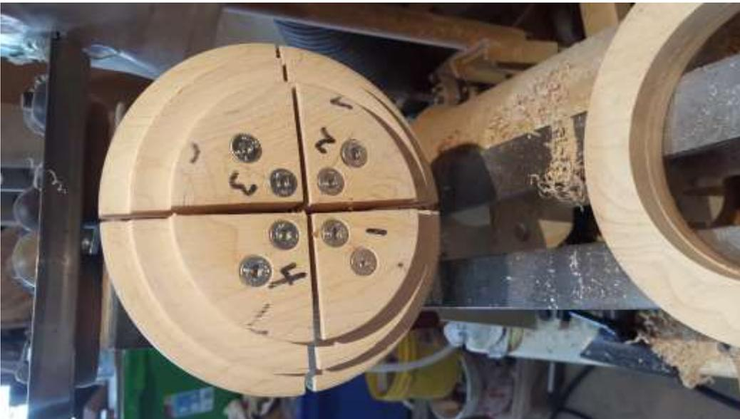
Place the top onto the step jaws.
