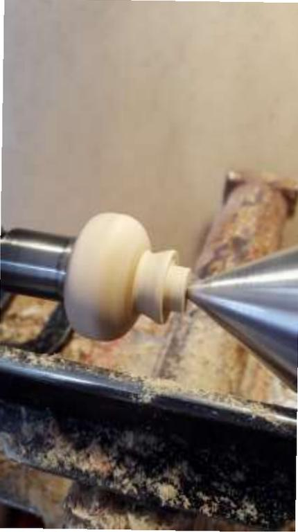
Use a Step type center drive and form the 1/2" inch or 9/16 inch tennon at the tailstock end. Sand the knob as needed for a good smooth finish.
