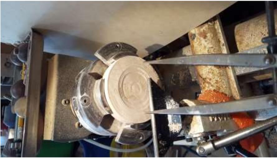
Turn the recess in the face of the disk, make sure that the cork fits and then sand the face smooth.
