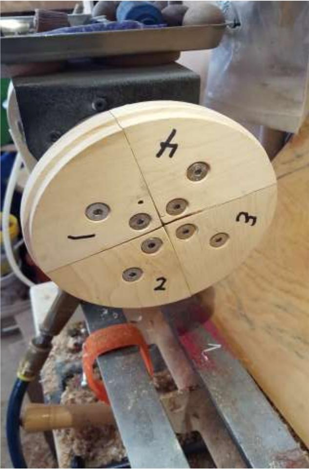
I have cut steps in the jaws of the Oneway Talon chuck allowing me to mount the top to clean up the inside. More on this later.
