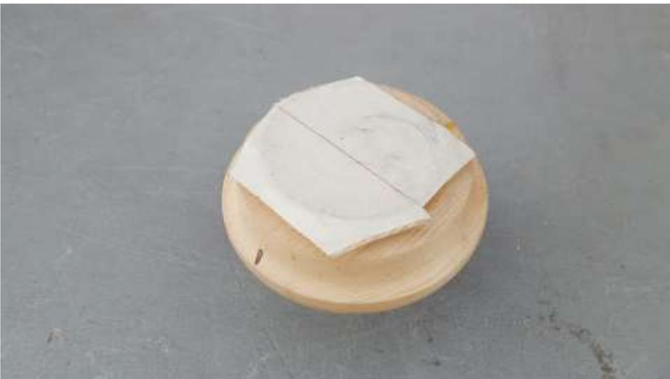
Use hot melt glue to hold the lid to the wood fastened to a metal faceplate. Again keep the tailstock in place until there is only a small nub left.
