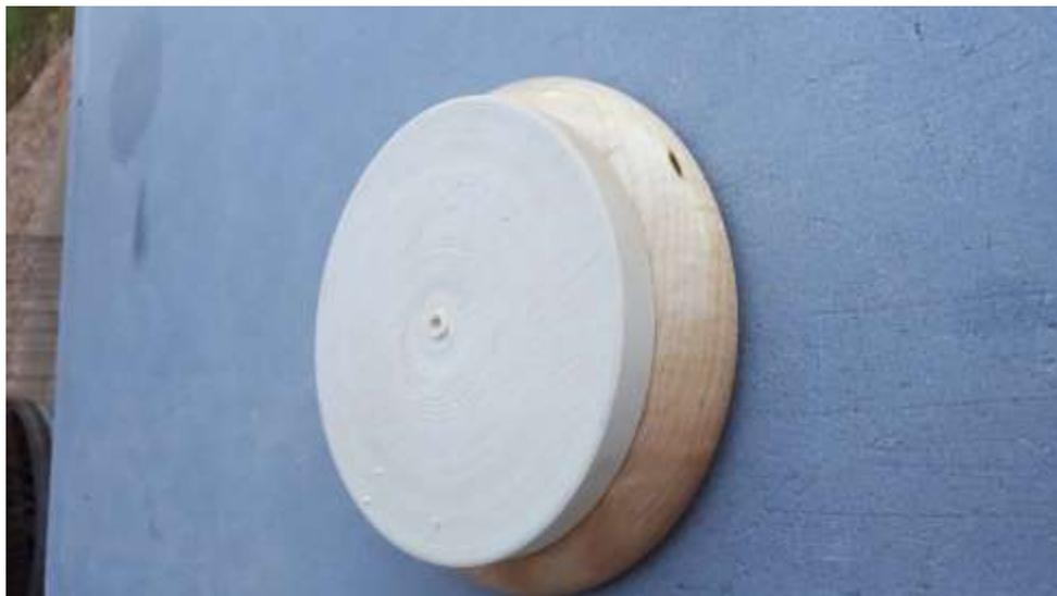
Lid is held in the chuck, formed, sanded and 1/2-inch hole drilled for the top knob. You may drill a 9/16-inch hole for the knob if you wish. I just got used to the 1/2" tennon for my knobs which will be discussed later.
