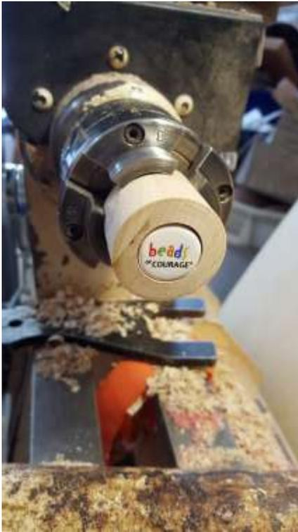
Form the top of the knob and sand using all the grits needed for a smooth finish.
