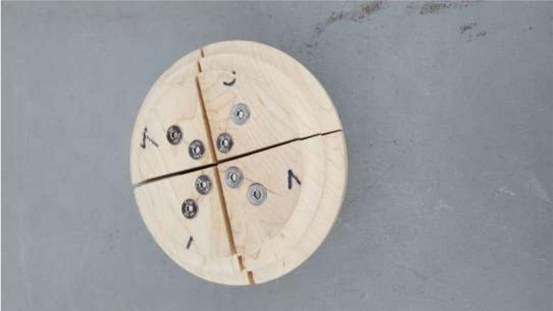
I have made much larger wooden jaws to hold the top and bottom pieces for the BOC boxes. You can do this if you do not have the Jumbo type aluminum jaws.
