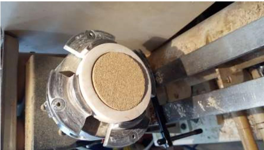
Turn the disk around and true up the bottom, sand smooth and if desired put a couple signature grove into the bottom.
