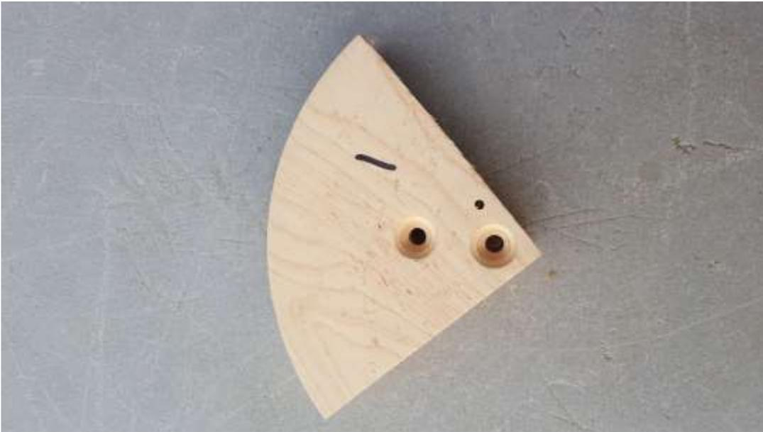
Place the drilled blanks onto the chuck with the screws slightly loose. Tighten the chuck down then tighten all screws. This will help align the wood to the chuck.
