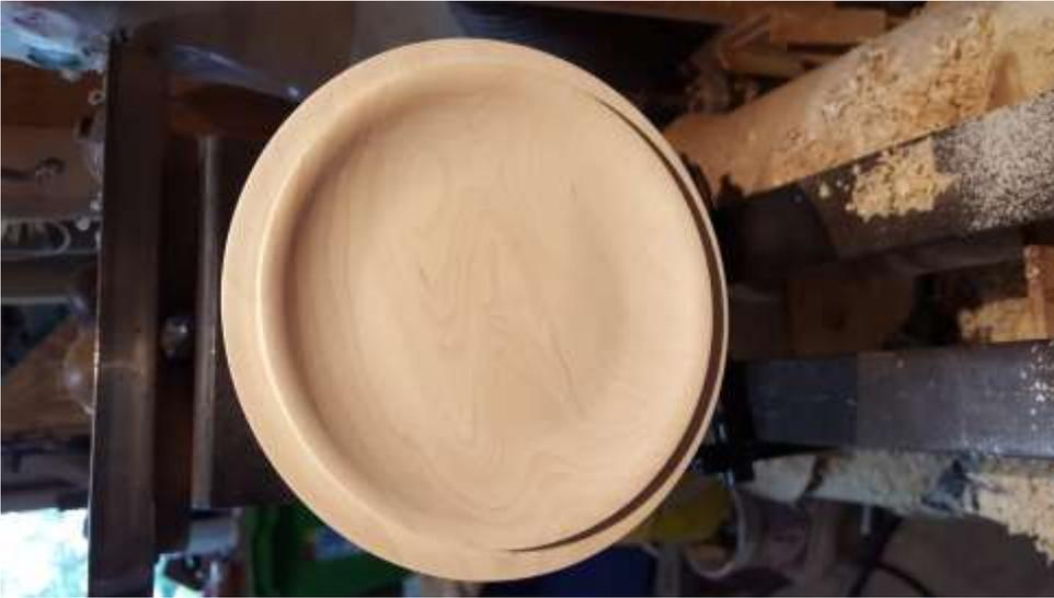
Note: I often use a vacuum system to turn the lid both the inside and the outside. I will turn the lid around and undercut the lid reducing the weight. If not using a vacuum system, you may do one of the following.
