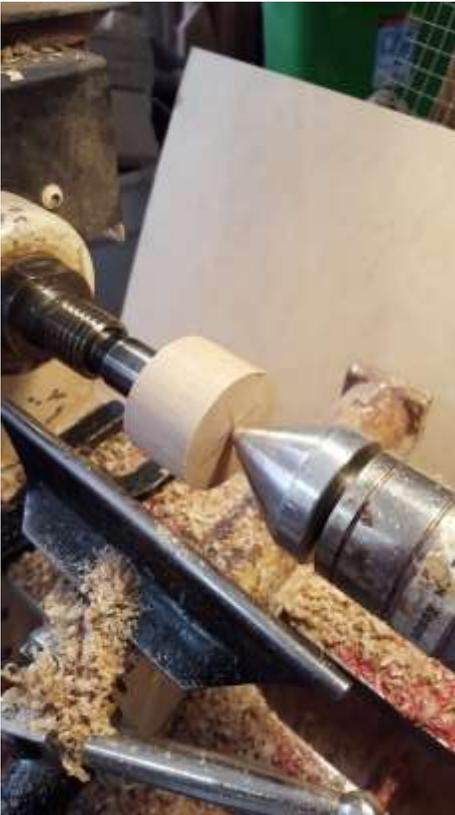
Place the blank into a small chuck, true up the tailstock side, drill a hole the size and depth for the BOC bead being used.
